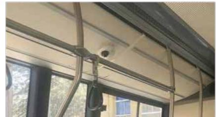
Each bus was fitted with 5-8 IP cameras located on the interior and exterior. The cameras provide a wider angle of view for safer driving, and can easily collect evidence when accidents occur.
