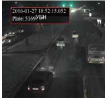
At 8 intersections, the E-police system took snapshots of violations. The system synchronizes the triggering signal to cameras when the signal detector detects red light signals. The Dahua all-in-one capture camera will take 3 images recorded of the violation, 1 image cutout of vehicle plate, status of the traffic signal, and plate number as violation evidence.
