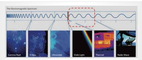
• Any object with a temperature above absolute zero(-273.15 °C) emits infrared radiation. Infrared radiation sits between the visible spectrum( $0.4^{\circ}0.75\mu m$ ) and microwave spectrum(>15 $\mu m$ ).
