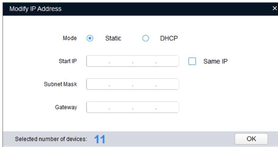
**Step 4** Select **Static** mode and enter start IP, subnet mask and gateway.
