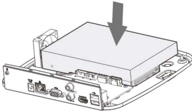
**Step 4** Turn the device upside down, match the screws with the holes on the HDD and then fasten them. The HDD is fixed to the baseboard.
