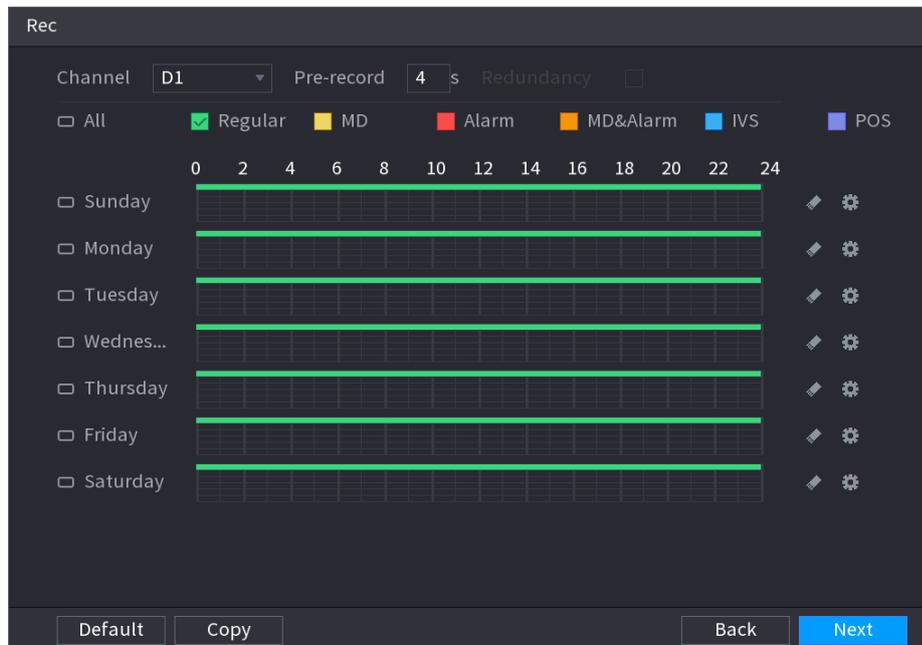
**Step 2** Configure parameters such as channel, pre-record, ANR and record type.
