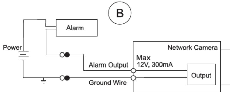
**Step 3** Log in web interface, and configure alarm input and alarm output in alarm setting.
