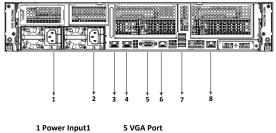
2 Power Input2 3 LAN Port1 4 LAN Port2 5 VGA Port 6 Serial Port 7 3\*USB3.0 Port 8 Management Port
