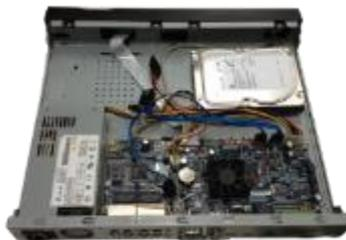
Step 3 Turn the device upside down and then secure the screws firmly. It is to fix the HDD on the chassis.
