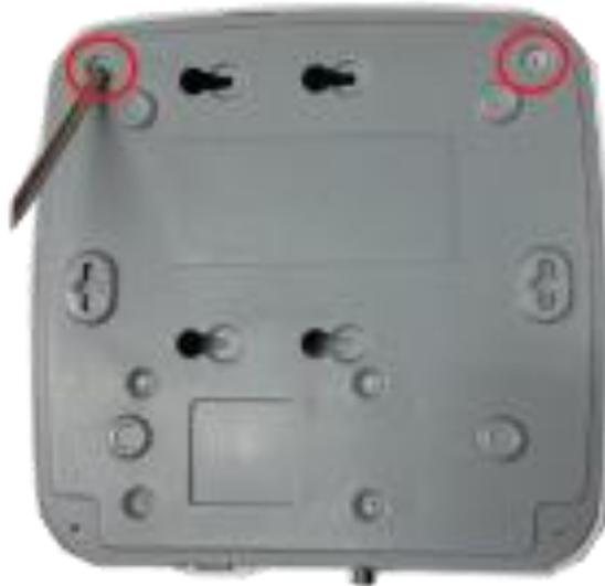
Step 2 Place the HDD in accordance with the four holes in the bottom.
