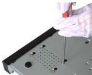
Step 6 Put the cover in accordance with the clip and then fix the screws on the rear panel and side panel.
