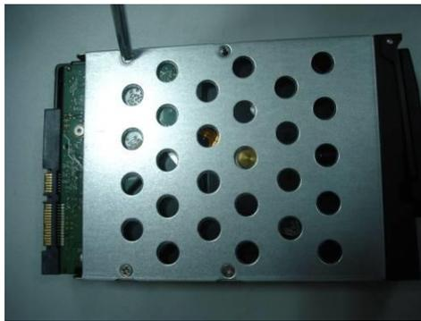
Step 2 Put the HDD to the HDD box at the front.
