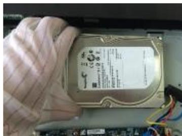
Step 5 Turn the device upside down; fix the screws to secure the HDD on the bottom of the chassis.
