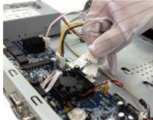
Step 3 Connect the other end of the HDD data cable and the power cable to the HDD.
