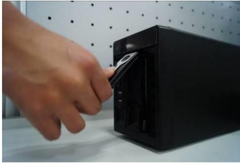
Step 4 Put the knob back after you insert the HDD to the SATA board.
