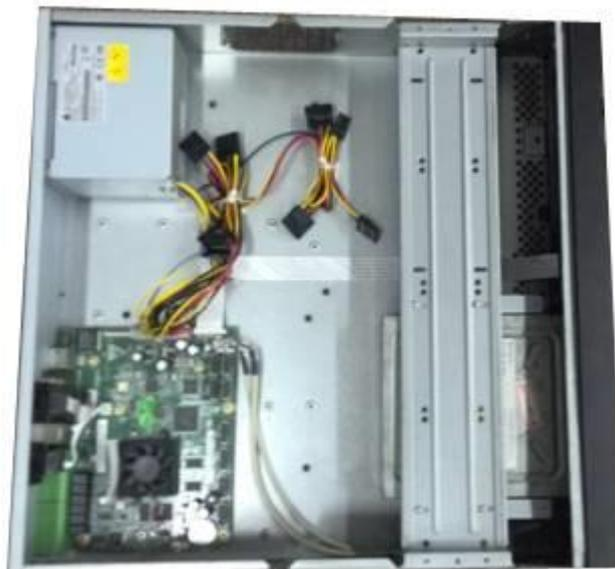
Step 8 Connect the SATA cable and power wire.
