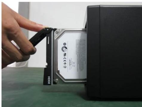
Step 3 Pull the HDD knob up when you put the HDD into the box in case the knob buckle may strike the front panel.
