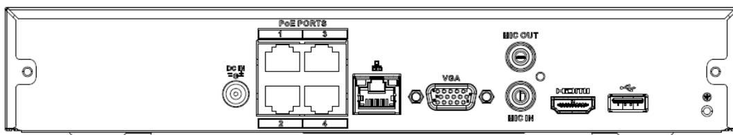
The NVR11HS-8P-S3H/21HS-8P-S2/21HS-8P-4KS2 series rear panel is shown as below. See Figure 2-30.
