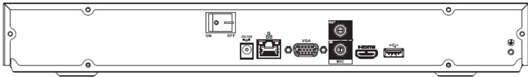
The NVR22-P-S2/22-P-4KS2 series rear panel is shown as below. See Figure 2-33.
