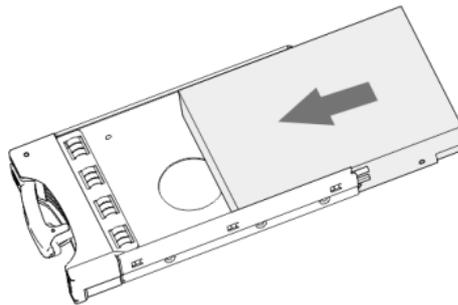
Step 3 Fix the disk in the drive tray with the four screws.
