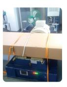
A walk-through metal detector is very heavy (max. 61kg). Sturdy packaging can help reduce damage during transit. We conduct drop and vibration tests to simulate package handling and road transportation, thus reducing the possibility of any damage.
